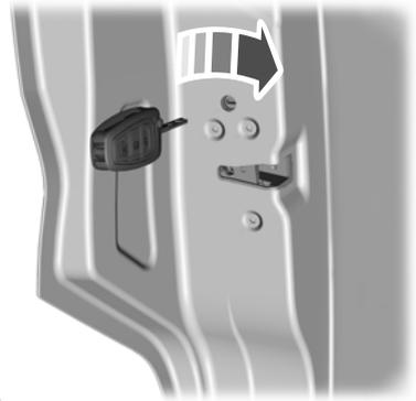
2. Insert the key blade into the key slot.
