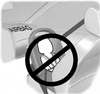
**WARNING:** Extreme Hazard! Never use a rearward facing child restraint on a seat protected by an active airbag in front of it. Death or serious injury to the child can occur.
